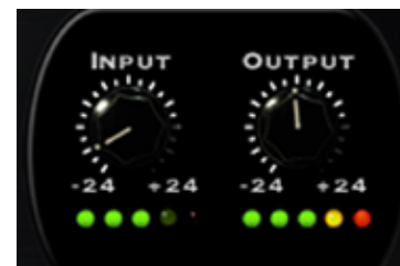
Figure 3: Output LED indicating maximum signal level
