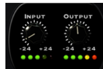
Figure 3: Output LED indicating maximum signal level
