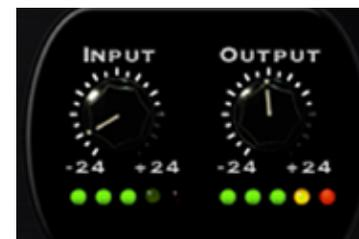
Figure 3: Output LED indicating maximum signal level
