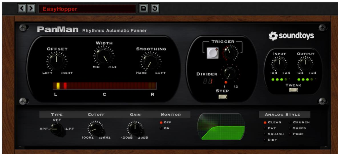
Figure 17: Step Mode's Control Panel and Tweak Menu
