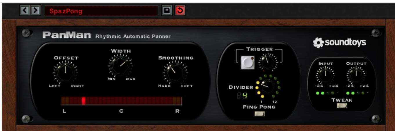
Figure 13: Control Layout in Ping Pong Mode
