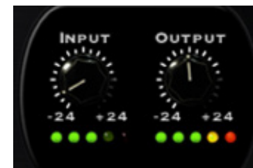
Figure 3: Output LED indicating maximum signal level
